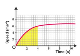
The shaded area represents the displacement of the car over a time period of 4 seconds. It can be calculated as:
